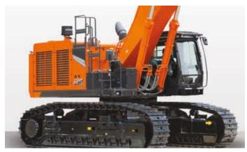
Access to the upper structure is easy via a new step.
