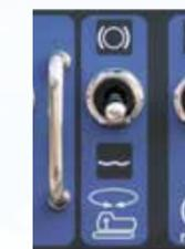
During work requiring the cab to swing (when the swing lever is in the neutral position), the operator may choose between free or brake mode depending on the work and personal preferences, making operations so much smoother.
