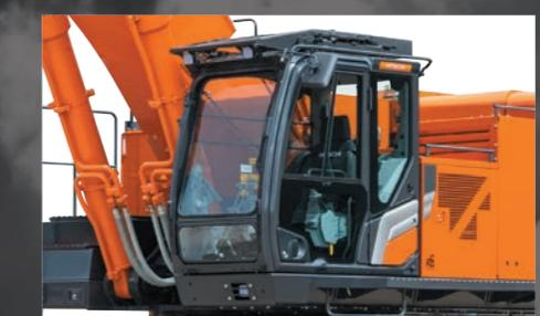
A reinforced cab for H&R specification machines with a reinforced windshield and a FOPS\* guard that protects the cab from falling objects. The front has a laminated straight glass front window that shuts out dust. The cab front guard (optional), also complies with the ISO standard OPG\*\*.
