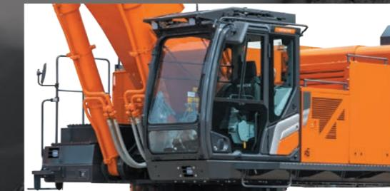
A reinforced cab for H&R specification machines with a reinforced windshield and a FOPS\* guard that protects the cab from falling objects. The front has a laminated straight glass front window that shuts out dust. The cab front guard (optional), also complies with the ISO standard OPG\*\*.
