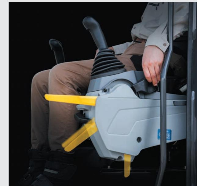
New designed pilot shut-off lever
