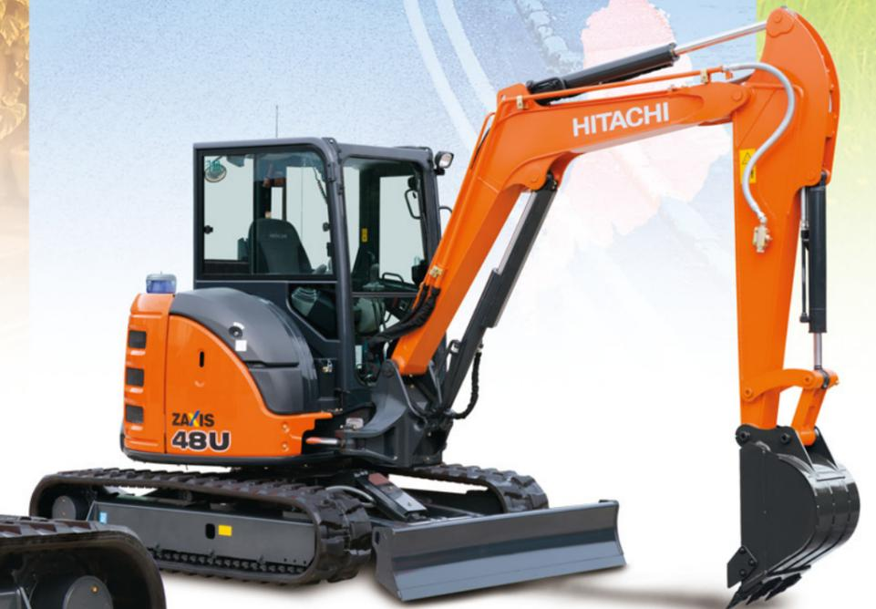
Shown equipped with 1.69 m arm, extra piping, additional counterweight, armrests, and auxiliary function lever as optional items.
