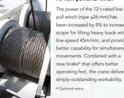
pull winch (rope  $_{\Phi}26$  mm) has been increased by 8% to increase scope for lifting heavy loads with line-speed 45m/min, and provide better capability for simultaneous movements. Combined with a new brake\* that offers better operating feel, the crane delivers simply outstanding workability. \* Optional extra
