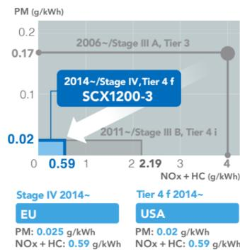
\* Compared with the SCX1200-2. Approximately 80% reduction in NOx emissions compared to the SCX1200-3 with previous engine (Stage III B/Tier 4 i).
