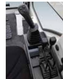
**Control levers with drum rotation sensor**
